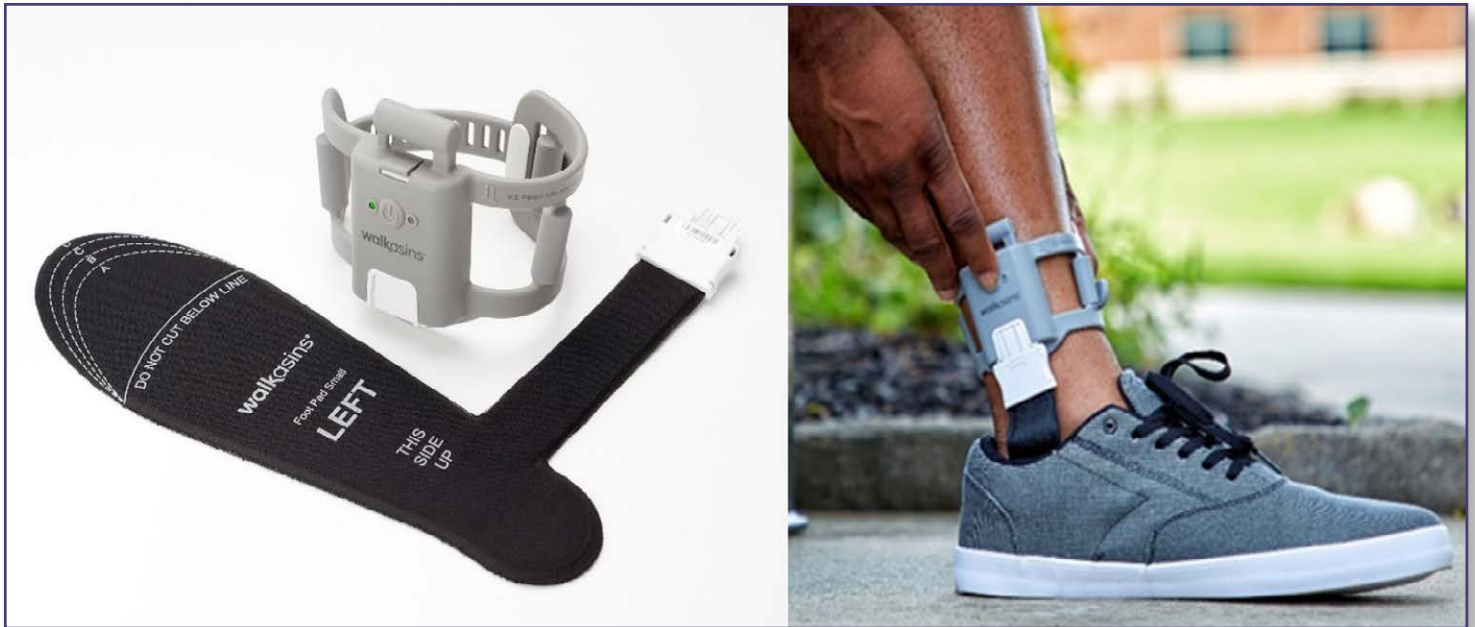
Figure 1. (Left) The two components of the Walkasins prosthetic device, the pressure sensitive flexible foot pad that is placed in the shoe and connects to the leg unit that contains a rechargeable battery, a microprocessor, supporting electronics, and four mechanical tactile stimulators. The embedded software algorithm evaluates pressure data and activates the mechanical tactile stimulators at relevant times during standing and walking to signal balance-related information to the afferent nervous system. (Right) A Walkasins user wearing the device in the process of turning it on. The Walkasins system is worn bilaterally (unilateral components depicted).
