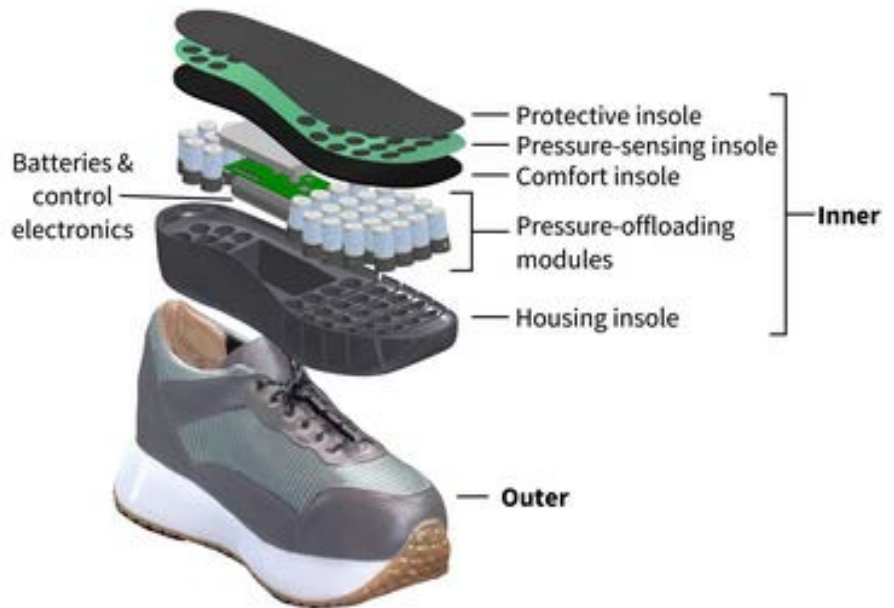
Figure 1. Schematic of the outer and inner (removable insole system) parts of the shoe.
