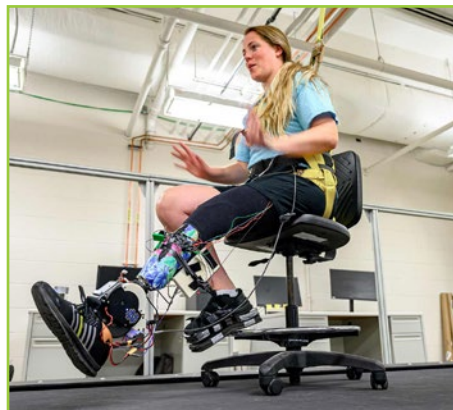
Light helps test out and give feedback on the powered prosthesis. Photograph courtesy of Notre Dame.
