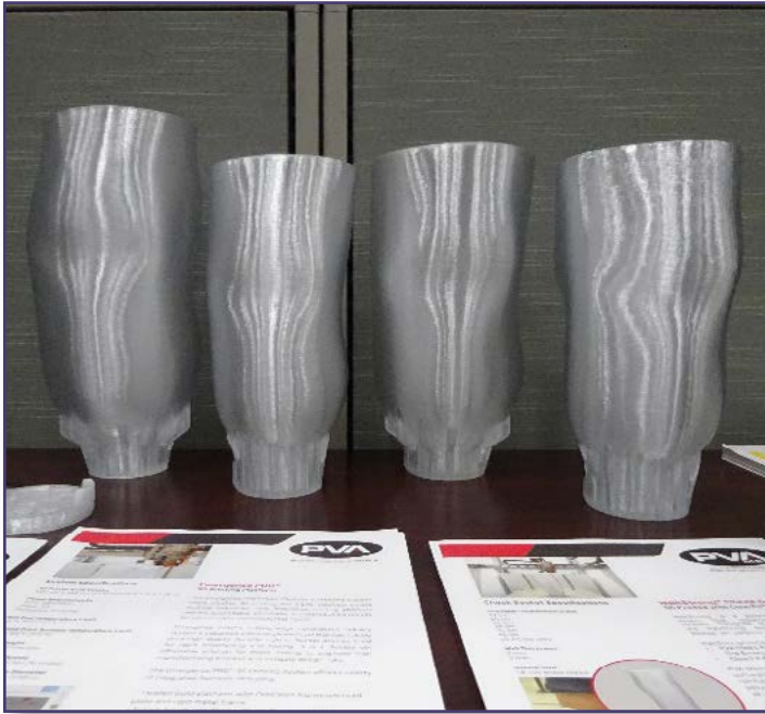
Samples of the Symphonie check socket product. Check sockets can be 3D printed in as little as 3–6 hours.
