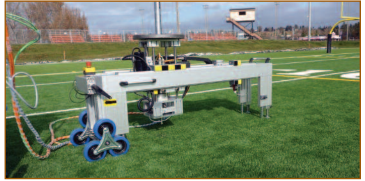
Figure 2. Photograph of the footwear traction tester performing a traction test on the field of play with the athlete's actual shoes used for competition.
