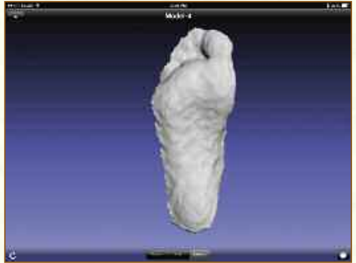
Some technologies in which a tablet-based scanning device is moved around the foot, such as those utilizing the 3D Occipital Structure Sensor (sample image at right), approach the accuracy of more conventional laser scanners.
